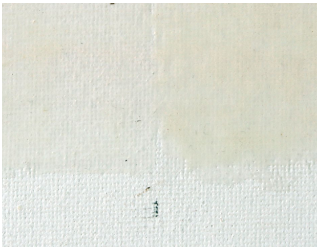
Figure 7. The effect of the reference varnish – colour and coating of the structure of the canvas – in one layer (left) and in two layers (right).
