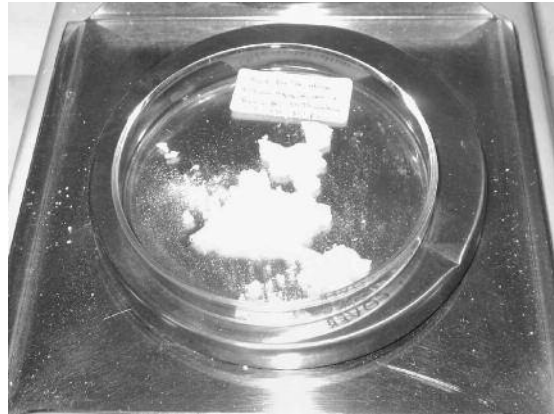
Fig. 2 Residue after drying of limewater additivated with metakaolin.
