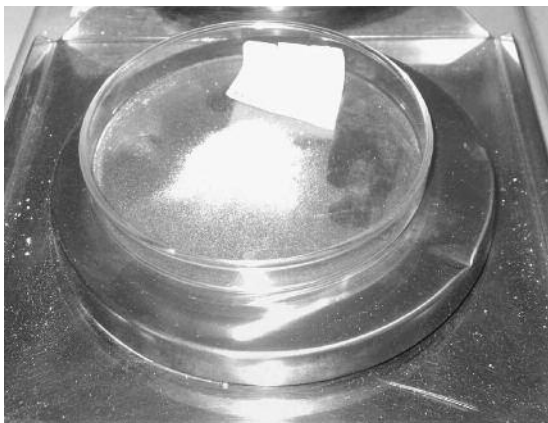
Fig. 1 Residue after drying of the simple limewater.
