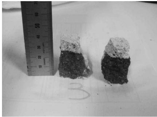
Fig. 4 Test for evaluation of consolidation deepness with phenolphthalein agent.
